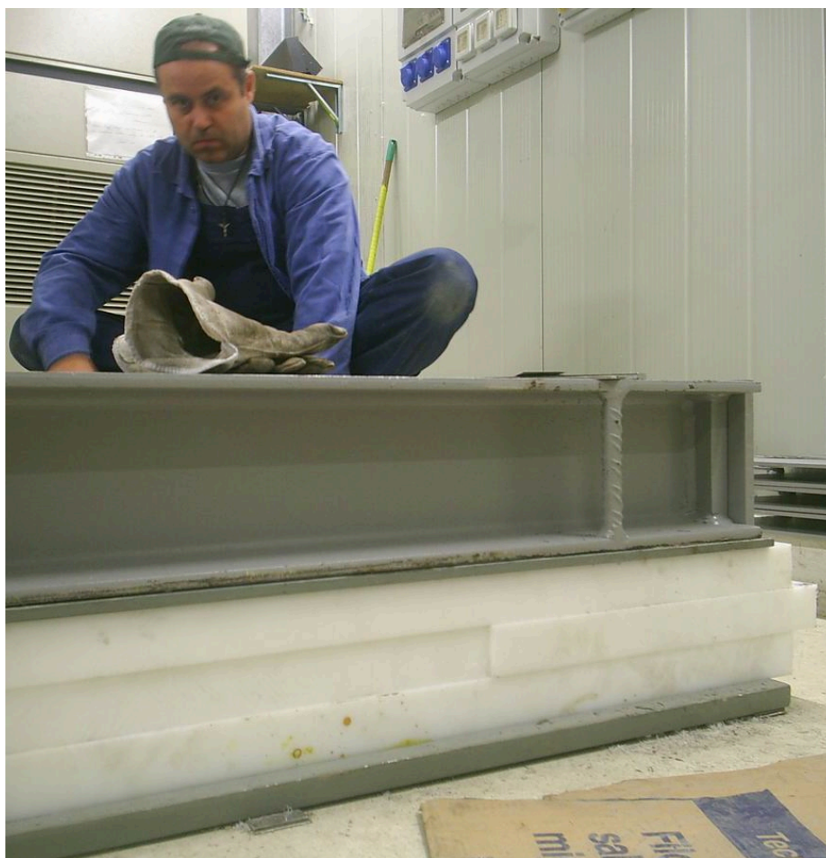
Figure 3.11: The entire shield was constructed on a 15 cm platform of high molecular weight polyethylene (“PE500”), which was structurally supported (sandwiched) by steel plates. The surface was leveled with steel shims. This was a precautionary step to ensure that neutrons could not be a limiting source of background. In contrast, additional shielding on the other 5 sides could have been added (but was not) as an after thought. The contractors were not always pleased by our exacting design requirements. This photo was taken shortly after discussing the requirements for cleaning all internal surfaces prior to installation. One of the more polite responses was “non ci credo!”
