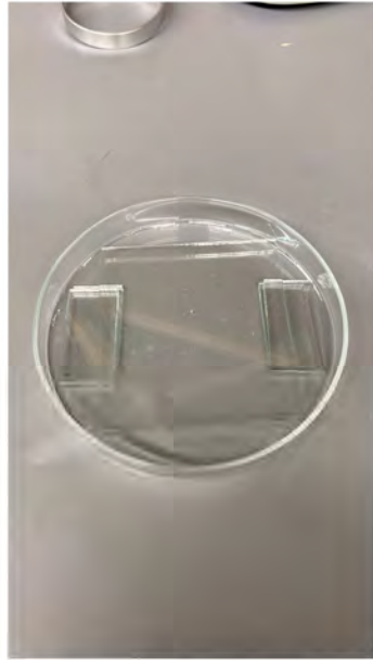
(a) Large set up for making shape memory polymer sheets
