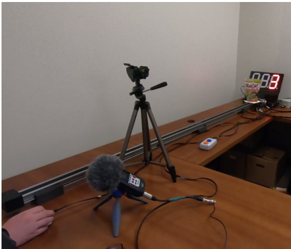
Figure 5. Conveyor Belt Provocation Task Setup. This is the setup of the Conveyor Belt Task at Baylor University as a part of the ABOVE study. The object in this image is placed at the farthest position from the participant. The readout board at the end shows the participant what they are rating when turning a rotary-encoder based dial.
