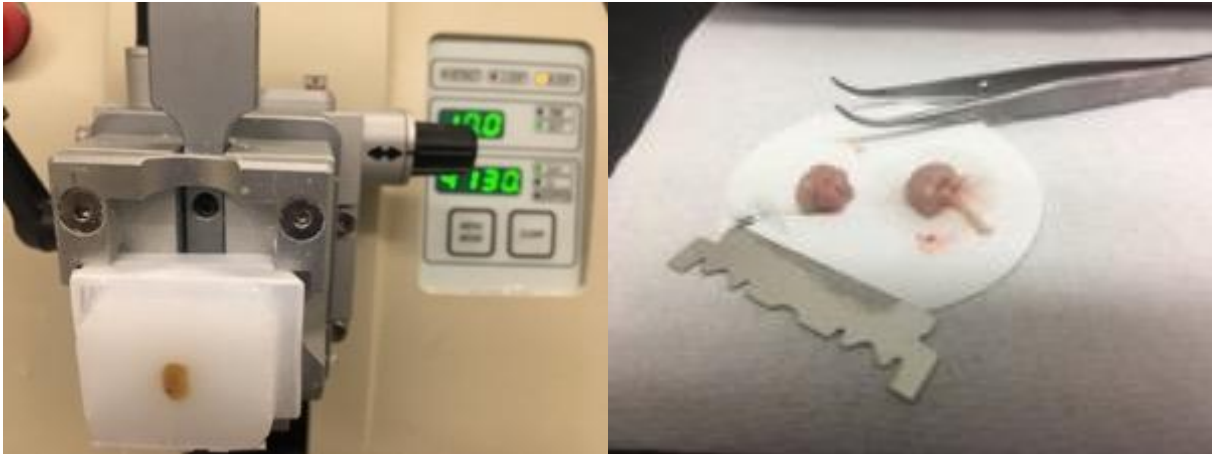
Figure 2. Left: Example of a paraffin-embedded-tissue cassette in place for microtome sectioning. Right: Example of live tissue at 4°C being sectioned coronally using half of a double-edge razor.
