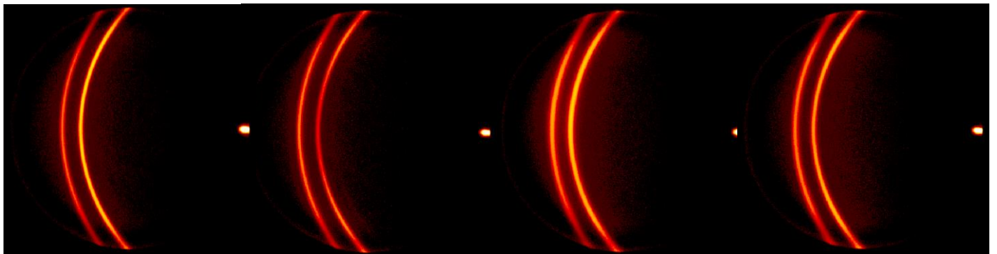
Figure 14. XRD scans of polyethylene samples unprocessed or processed at 30°C, 50°C, or 60°C.
