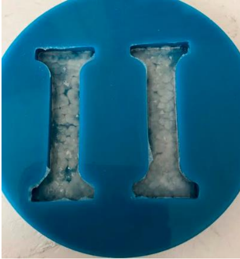
Figure 18. Samples drying after oven into dogbone shapes
