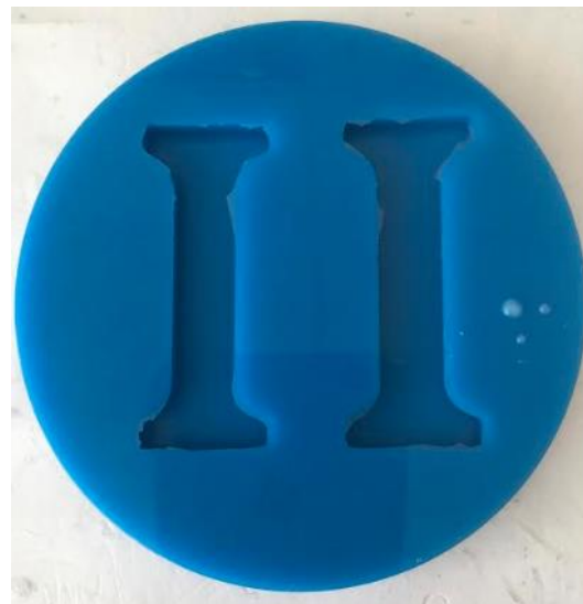
Figure 11. Silicon Mold used to create dogbone Instron samples
