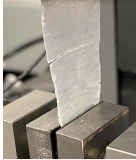
Figure 19. Sample processed at 55°C breaking after tensile test in Instron
