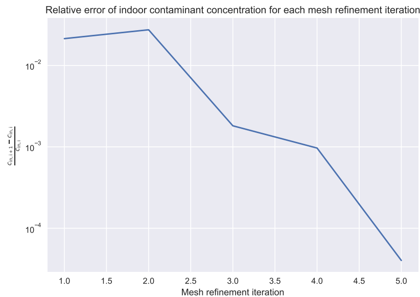
Figure 2.13: Convergence of indoor air contaminant concentration as the mesh is refined.
