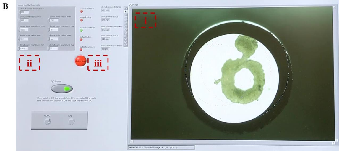
Supplemental Figure 3.4 Real-time tissue ring quality control. Screenshots of the custom LabVIEW algorithm performing quality control on two tissue rings. The first panel shows QC of a tissue ring (i) that passes, with the center distance, inner radius, inner roundness, outer radius and outer roundness parameters measured within the given range (ii). The read-out lights for each parameter are green, and the overall read-out light is green (iii) (A). The second panel shows QC of a tissue ring (i) that fails, with center distance, inner radius, outer radius and outer roundness parameters measured outside the given range (ii). The read-out lights for the failed parameters are red, and the overall read-out light is red (iii) (B).
