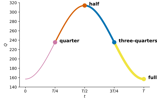
Figure 5.6: Time-dependent boundary condition for the simple fluid example. The volume-fluxes ( Q ) at the boundaries are prescribed as a sinusoidal function of time. The peak Q for the parent pipe is 314 as shown here. Since each daughter pipes has a volume-flux half of that of the parent pipe, its peak Q is 175. The temporal space, a full sinusoidal period, is divided into four quarters. The end of each quarter is marked on the plot.
