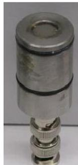
Figure 80: Polyvinylidene fluoride (PVDF) film transducer.
