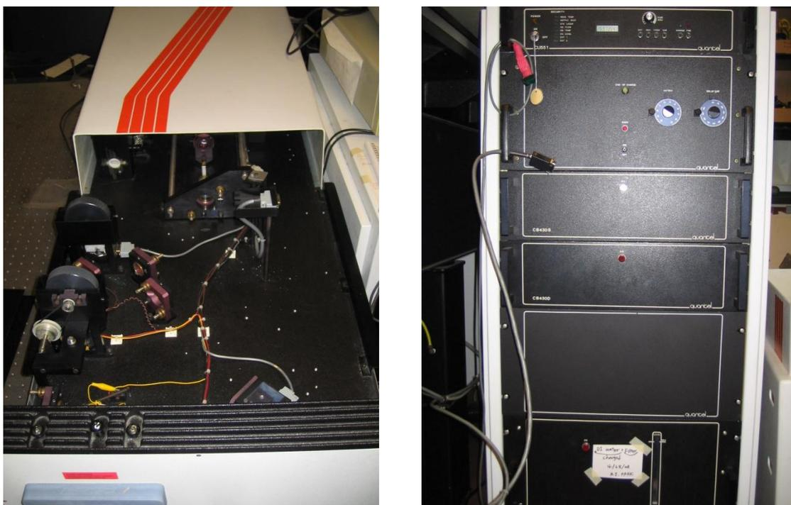
Figure 66: Actively Q-switched Nd:YAG laser (YG 580 series, Quantel International).
