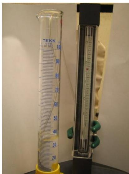
Figure 56: Experimental setup for Sparging. A flowmeter is shown as well.
