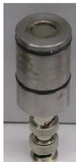
Figure 80: Polyvinylidene fluoride (PVDF) film transducer.
