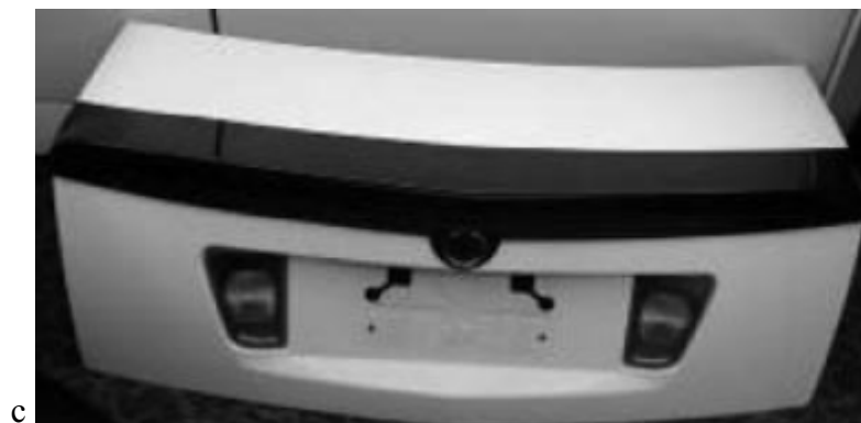
Figure 1.9: A decklid assembly for the Cadillac STS . (a) The decklid inner panel formed from magnesium AZ31B. (b) The decklid assembly from the inside. The inner panel is painted black. (c) The decklid assembly from the outside. The outer panel is made of hot blow formed aluminum alloy 5083. The spoiler is a polymeric material. (Carter, Krajewski, et al., 2008).
