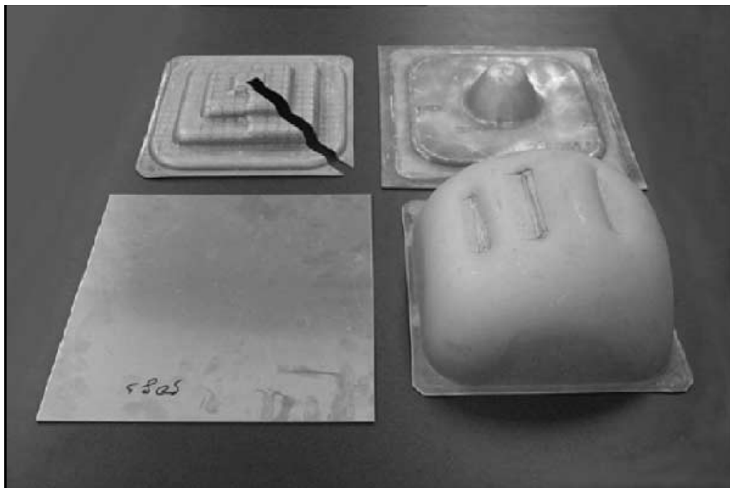
Figure 1.4: Complex parts formed from an aluminum alloy using superplastic forming processes (Chandra, 2002).
