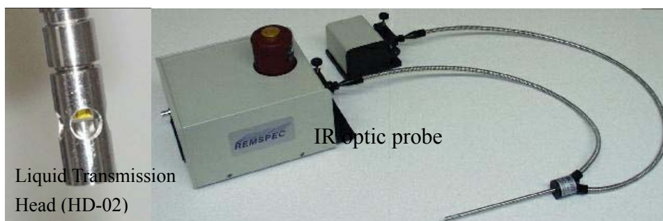
Figure 2-4. In-situ IR probe with external detector and its tip 2
