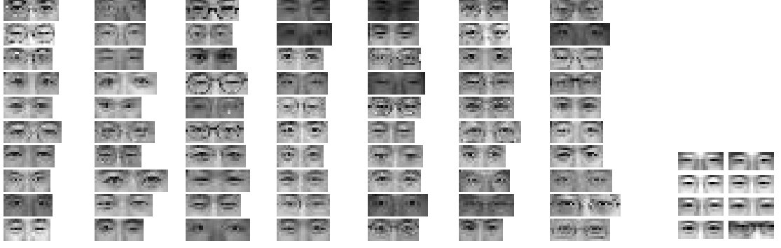
Figure 4.14: The left panel shows 70 East Asian eyes, each with height of 10 pixels. The right panel shows the 8 templates, each with size 8 \times 20 , learned from the model with mixtures over 4 scales: 1.2, 1.1, 1, and 0.9.
