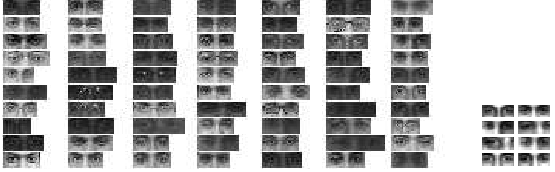
Figure 4.15: The left panel shows 70 Indian eyes, each with height of 10 pixels. The right panel shows the 8 templates, each with size 8 \times 20 , learned from the model with mixtures over 4 scales: 1.2, 1.1, 1, and 0.9.
