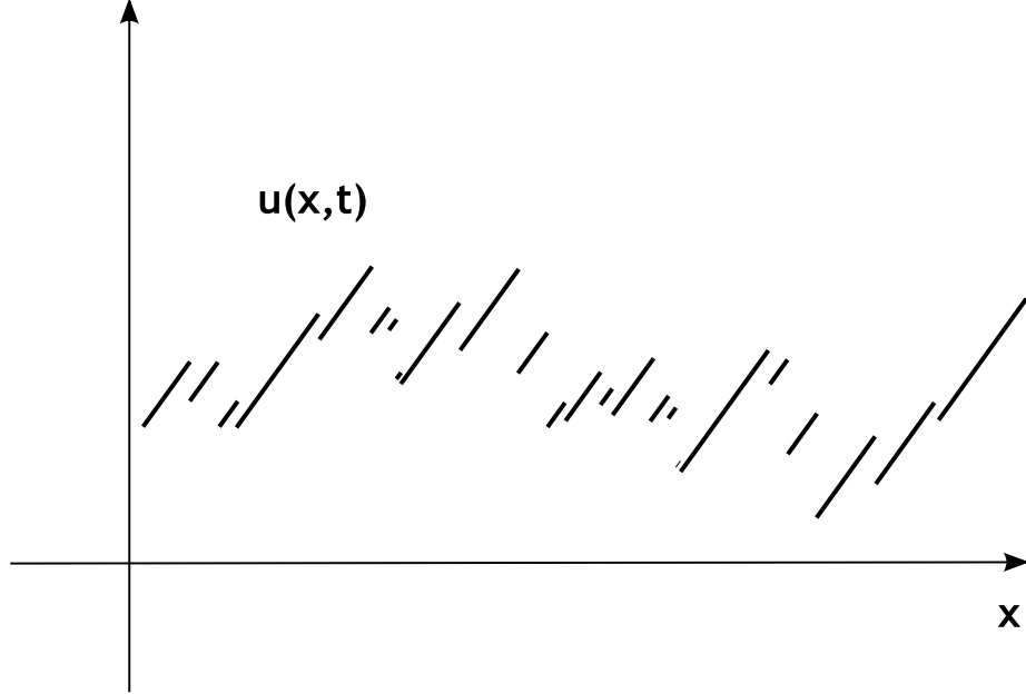
FIGURE 1.1. Typical sawtooth profile of a solution u(x, t) to the inviscid Burgers equation. The ramp-like structures have slope t^{-1} and are interspersed with shocks that undergo ballistic aggregation.
