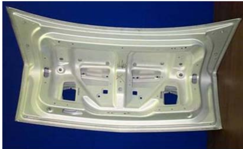
Figure 1-2 Deck lid of Cadillac STS car made using the QPF process. (a) inner panel, and (b) outer panel. Inner and outer panels are hemmed together to make the assembly panel. Courtesy of General Motors R&D Center.
