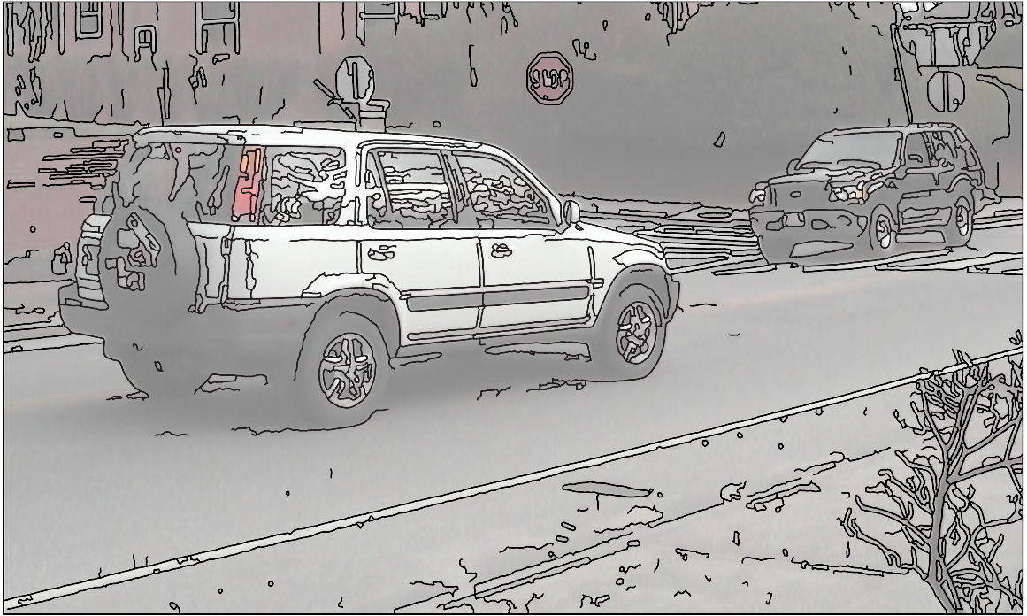
Figure 2.6: Curves detected and overlaid on the vehicle image from Figure 2.1. Edge are detected with a variation of the Canny detector, estimated to sub-pixel location with parabolic interpolation, and linked into curves.
