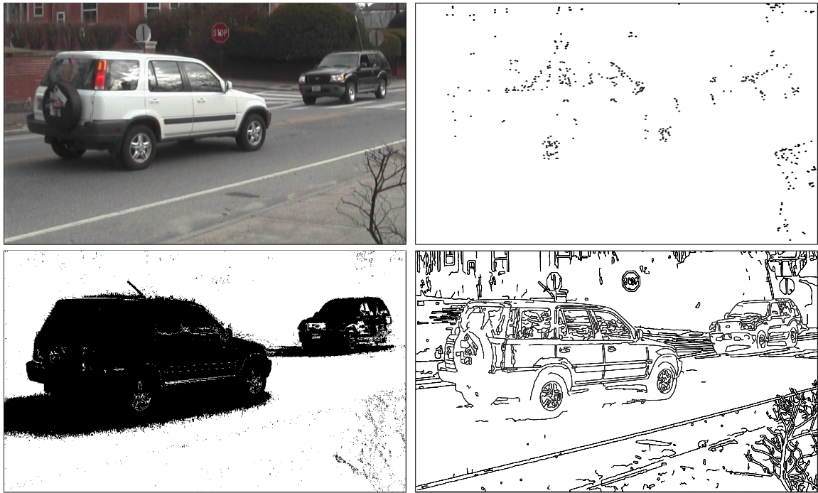
Figure 2.4: Geometric features of varying intrinsic dimension. Clockwise from upper left: the original image, detected points (Harris corners), detected curves (sub-pixel Canny edges), detected regions (Stauffer-Grimson foreground regions).
