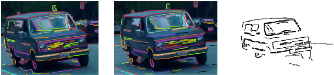
Figure 2.10: Tracked 2-d curves. The left two images show matching curves (color coded by match). The right most image shows vehicle curves segmented from the background by common motion. Images adapted from Figures 11 and 13 of [52].
