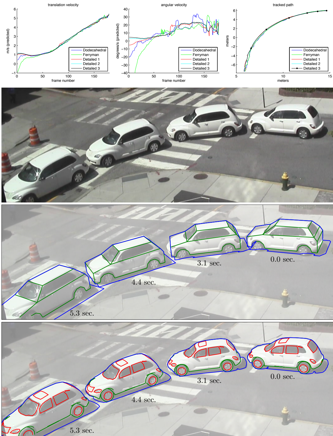
Figure 8.2: Tracking a white PT Cruiser with fixed shape models in pole view. Plots show estimated translation velocity, angular velocity, and path for all models. The top image is a montage of four key frames. The middle and bottom images overlay Ferryman and Detailed 3 results, respectively.
