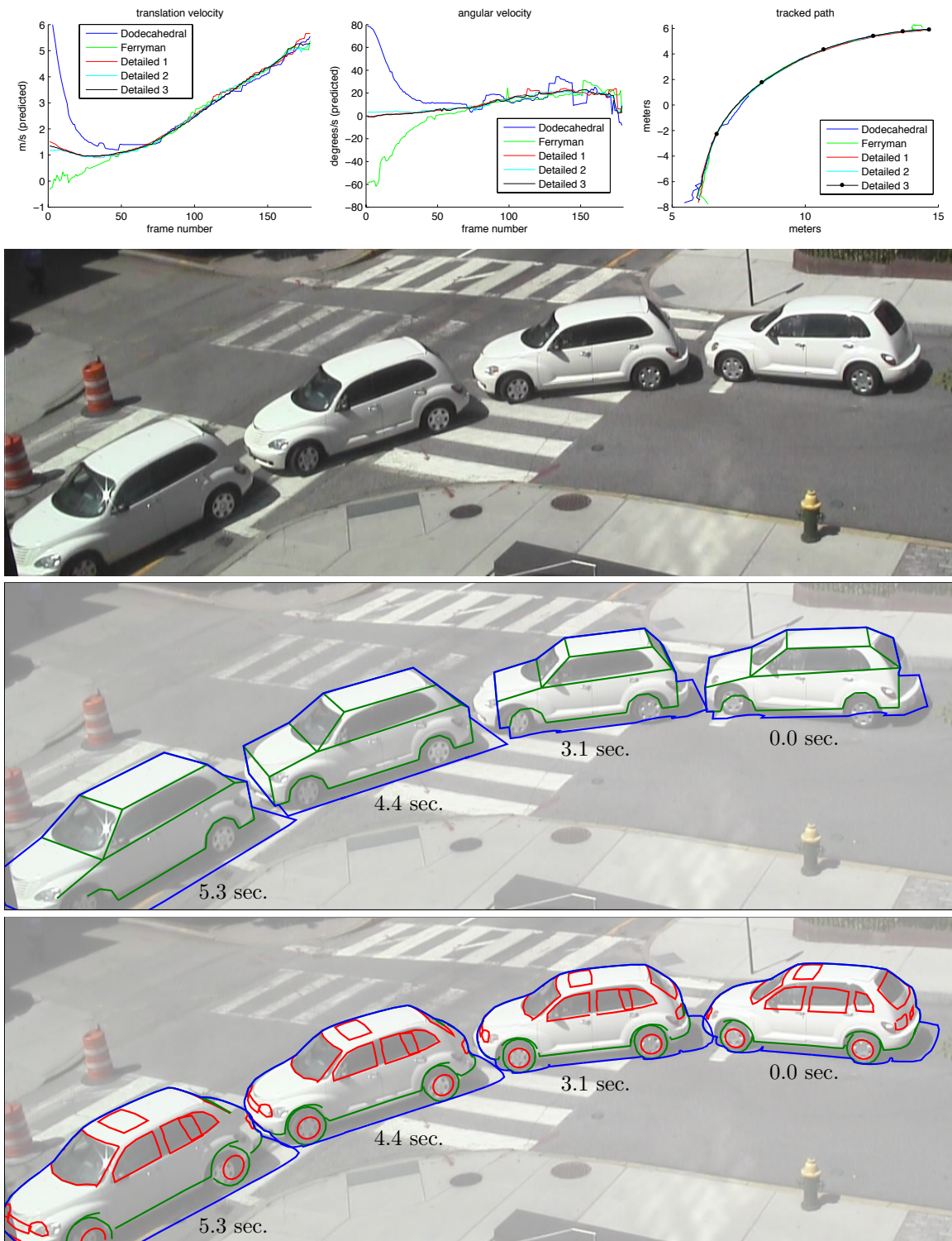
Figure 8.5: Tracking a white PT Cruiser with variable shape models in pole view. Results are directly comparable with Figure 8.2. The only difference is the addition of shape estimation.
