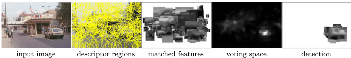
Figure 2.13: Code book vehicle detection. Points with descriptors are detected, matched to a code book, and then vote for vehicle center. Images adapted from Figure 5 of [67].
