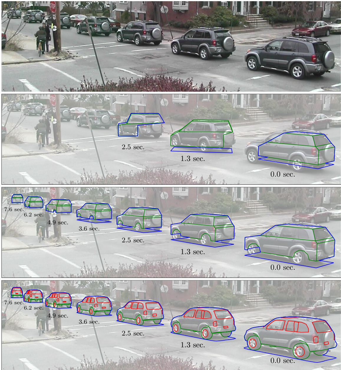
Figure 8.9: Tracking and shape estimation of a compact crossover SUV in ground view. This montage shows seven key frames. From top to bottom the overlays are Dodecahedral, Ferryman, and Detailed 3. The Dodecahedral model diverges in shape early on and loses track after 2.5 seconds.
