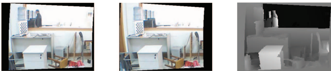
Figure 2.1: Stereo reconstruction input (two left-most images) and resulting depth map (right). Results and image taken from Wang and Zheng [70]
