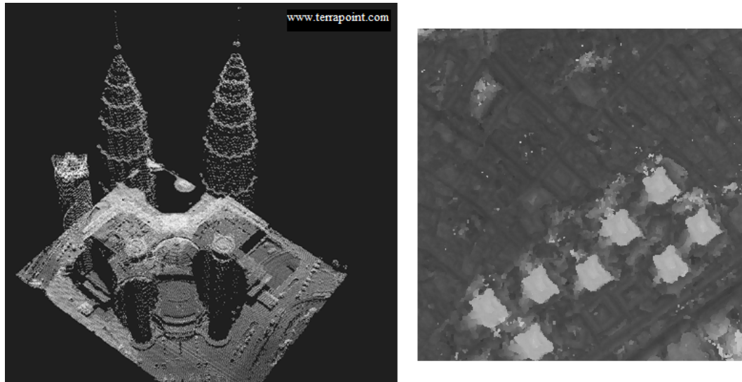
Figure 6.1: Two common forms of LIDAR are the raw point cloud output (left) and a processed digital elevation map (DEM) where brighter pixel intensities indicate taller structures (right). Left image copyright Ambercore Software, Inc.
