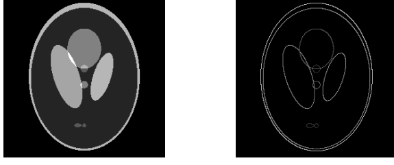
Figure 1.1: (Left) 256 \times 256 Sparse Gradient Shepp-Logan phantom image. (Right) Nonzero horizontal and vertical discrete gradient information.
