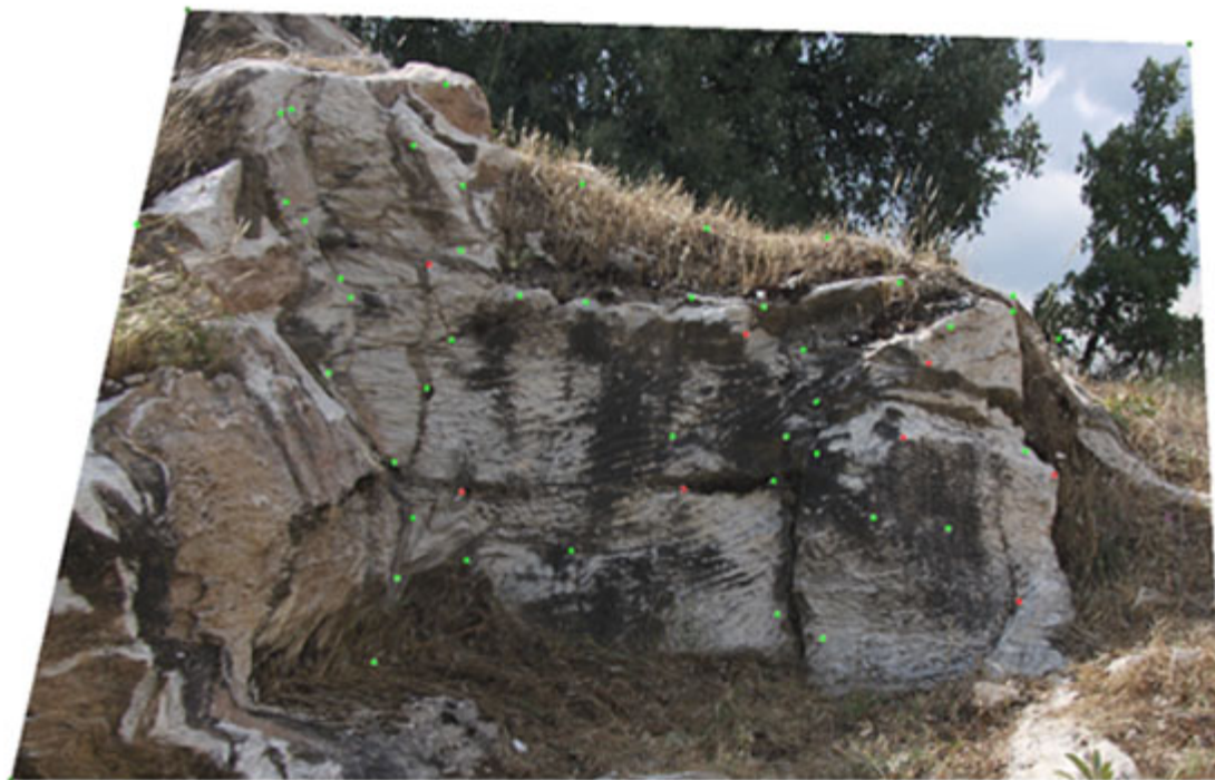
Figure 5.8: Photorectification points on quarry surface at Yeniköy 6. Green points are anchor points, while red points are topographic points (image created by John Valainis, courtesy of the Central Lydia Archaeological Survey).
