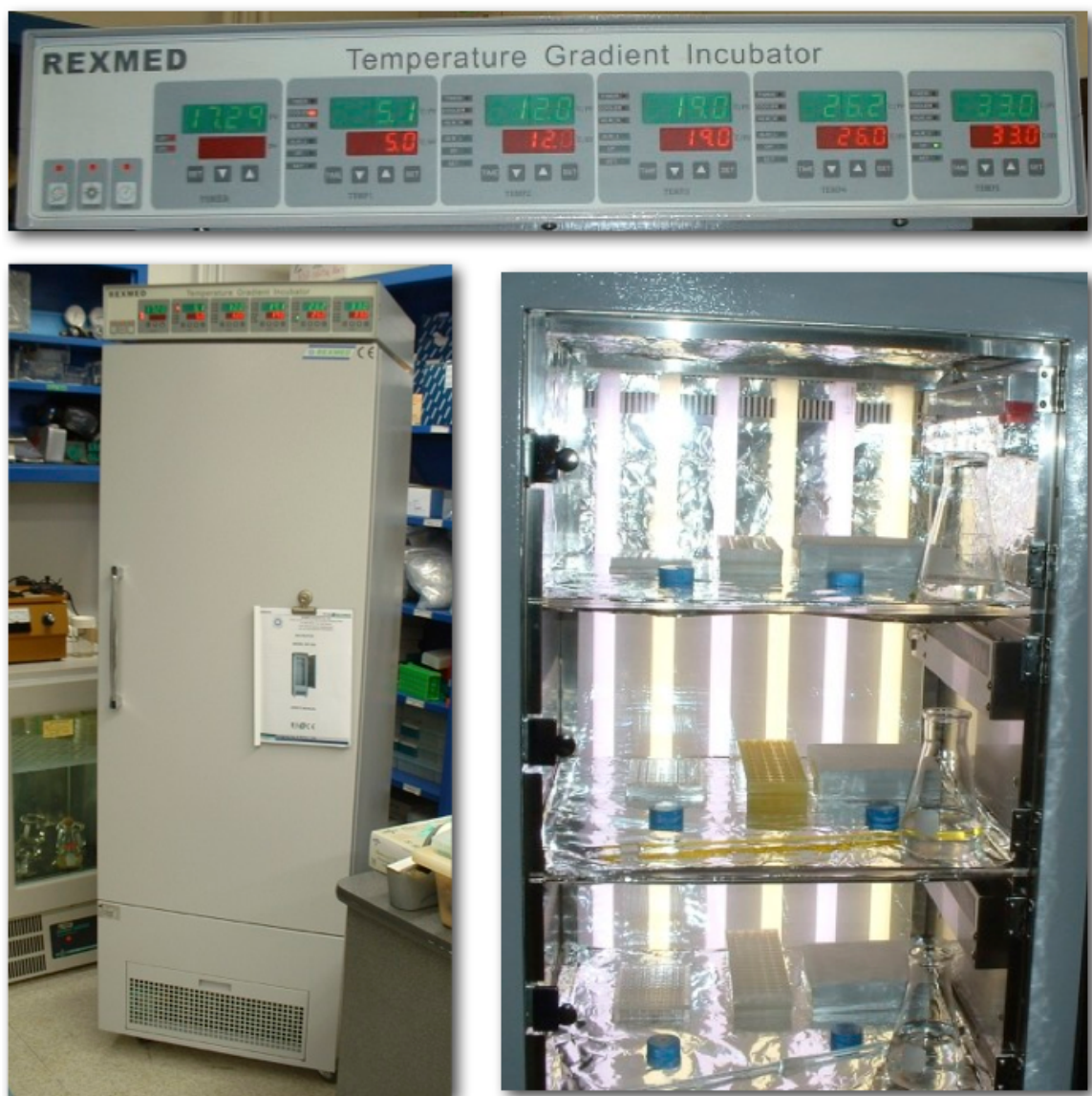
Fig. 2.5. The Rexmed RIT 450 (Rexmed Inc. Taiwan) gradient incubator. This was used as it has five compartments capable of each holding a different temperature. Aluminum foil was used to normalize the light in each chamber. The light cycle was a 16h:8h light/dark cycle and a mix of Philips TLD36W/840 (cool white) and Philips TLD36w (aqua) fluorescent light at 54 \pm 2 \mu\text{mol photons} \cdot \text{m}^{-2} \cdot \text{s}^{-1} as measured with a PAR detector (PMA2100/PMA2132, Solar Light Company, PA, USA).
