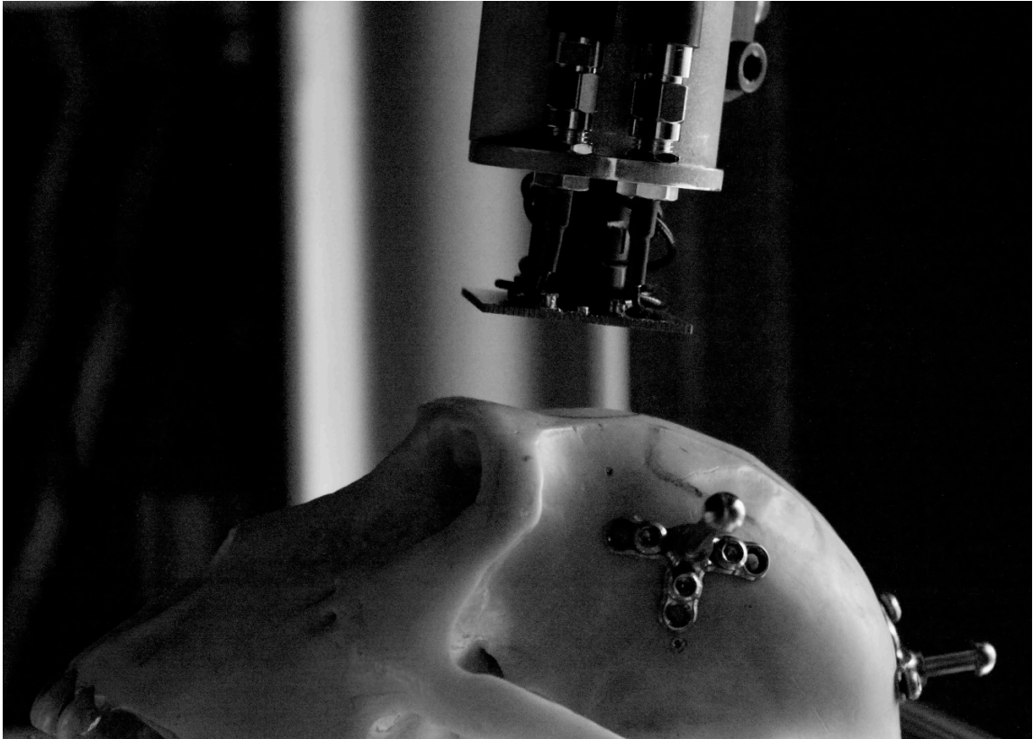
Figure 3-19: RF-IR transceiver positioned above a representative primate skull. The box is held by a 4-axis adjustable arm (x-y-z-pivot) for fine placement over the implanted microsystem. The photodiode resides inside the aluminum case to protect it from RF “noise” coming from the primary coil powering the microsystem. Two SMA connectors can be seen, which, deliver forward power and sense flux voltage going to the implant and are used to monitor power consumption of the system and safety.
