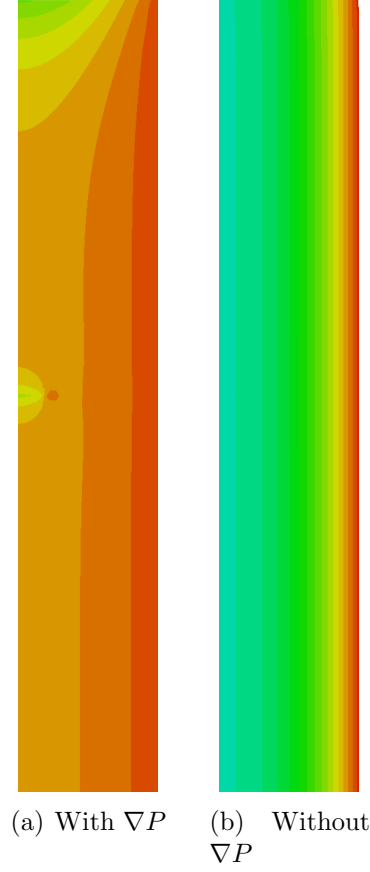
Figure 5.8: Concentration contours for a 350 nm nanowire charged at a rate of 3C , after being lithiated for 150 seconds. The contours represent the concentration distribution within the material with (a) and without (b) the pressure-gradient effects. The lowest level (blue) corresponds to zero and the highest level (red) corresponds to a concentration of 7.5 \times 10^{-3} \text{ mol/cm}^3 .
