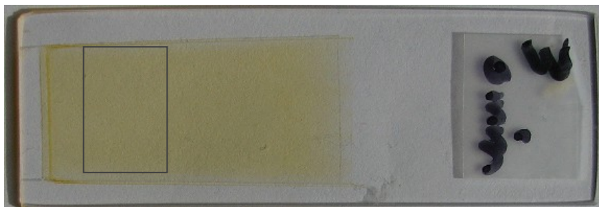
Figure 3.1. \beta -carotene containing film samples prepared on quartz slides. The rectangle is the area that was examined by the UV-vis spectrophotometer for photodegradation.
