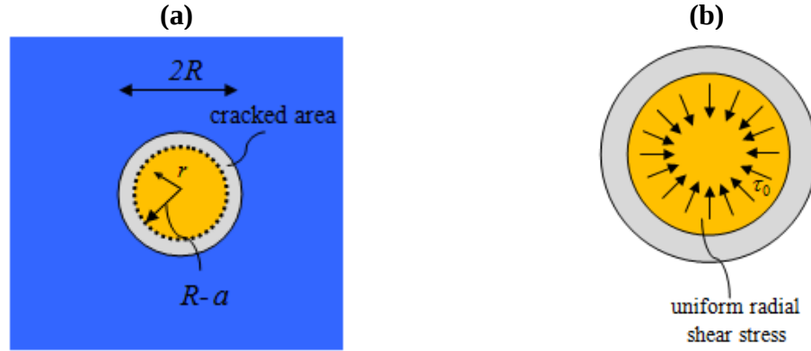
Figure 5.6: Schematic of (a) a Si circular island on substrate with an annular edge crack and (b) a free-body diagram of the island.
