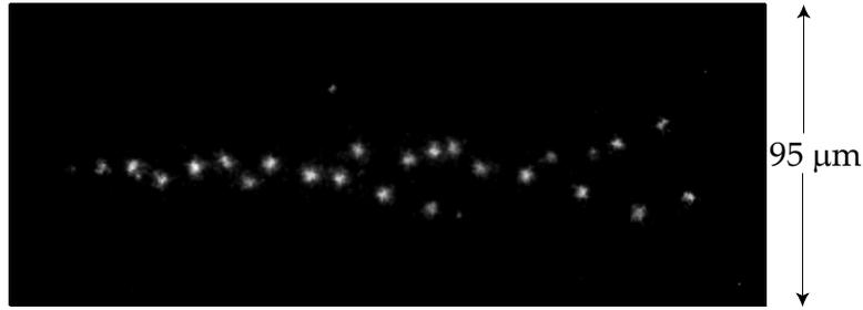
Figure 9.2: A single-exposure fluorescence image of the electro-spray droplets.
