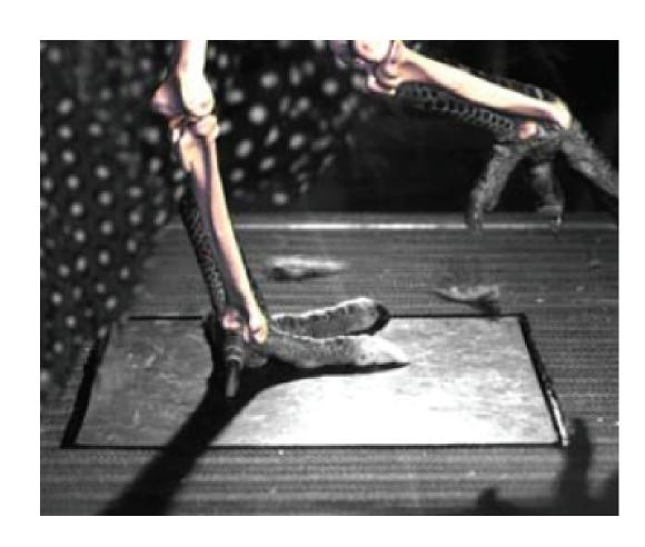
Synchronized force plate recordings were used to calculate the magnitude, position, and orientation of the ground reaction force (GRF). Mid-stance frames were sorted and analyzed based on bird speed and distance of the knee from the GRF. Attention was also paid to whether the bird was accelerating, decelerating, or moving at a steady pace during mid-stance.
