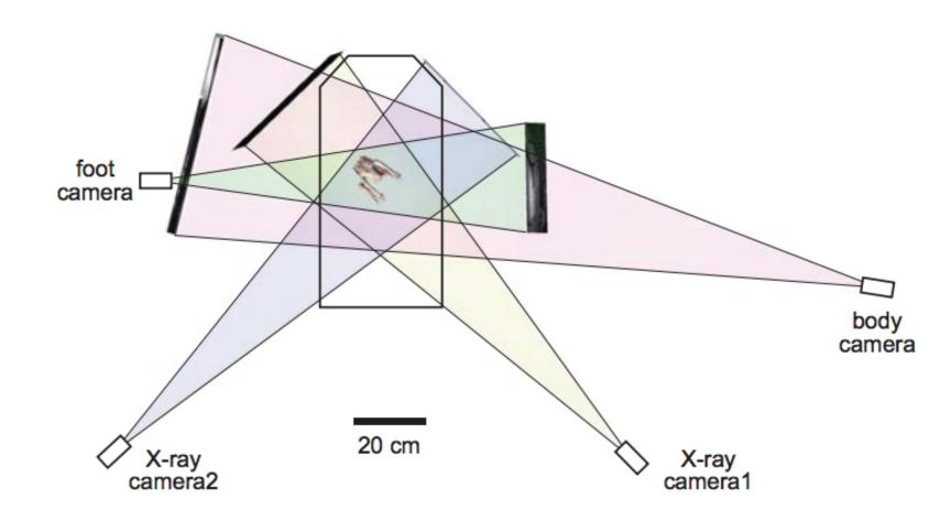
XROMM merges biplanar x-ray videos with bone models derived from CT scans, producing animations for accurately measuring 3D movement.
