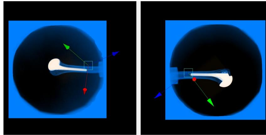
**Figure 2:** Autoscooper software combines bi-planar X-ray data from XROMM cameras 1 and 2 with 3D implant/bone model
