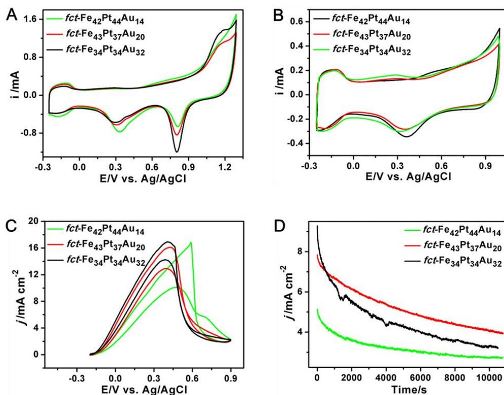
**Figure 7-6.** (A, B) CVs of the *fct*-FePtAu NPs with different compositions in the  $N_2$ -saturated 0.5 M  $H_2SO_4$  solution with the potentials scanned from -0.25 to 1.0 V (A) and -0.25 to 1.30 V (B). (C) *j*-*V* curves of the *fct*-FePtAu NPs with different compositions in the  $N_2$ -saturated 0.5 M  $H_2SO_4$  + 0.5 M  $HCOOH$  solutions. (D) *j*-*t* curves of the *fct*-FePtAu NPs with different compositions reflecting the specific activity change over time.
