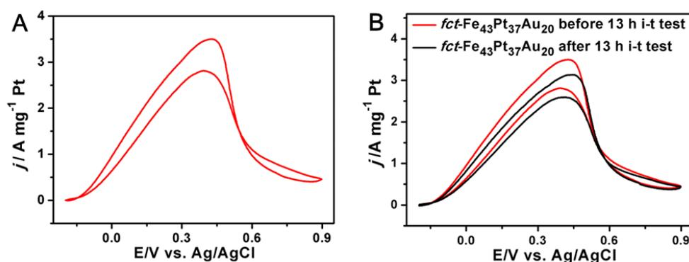
**Figure 7-9.** (A) *j*-V curves of the mass activity of the *fct*-Fe<sub>43</sub>Pt<sub>37</sub>Au<sub>20</sub> NPs; and (B) *j*-V curves of the *fct*-Fe<sub>43</sub>Pt<sub>37</sub>Au<sub>20</sub> NPs before and after 13 h *i*-*t* stability test. The studies were performed in the N<sub>2</sub>-saturated 0.5 M H<sub>2</sub>SO<sub>4</sub> + 0.5 M HCOOH solution.
