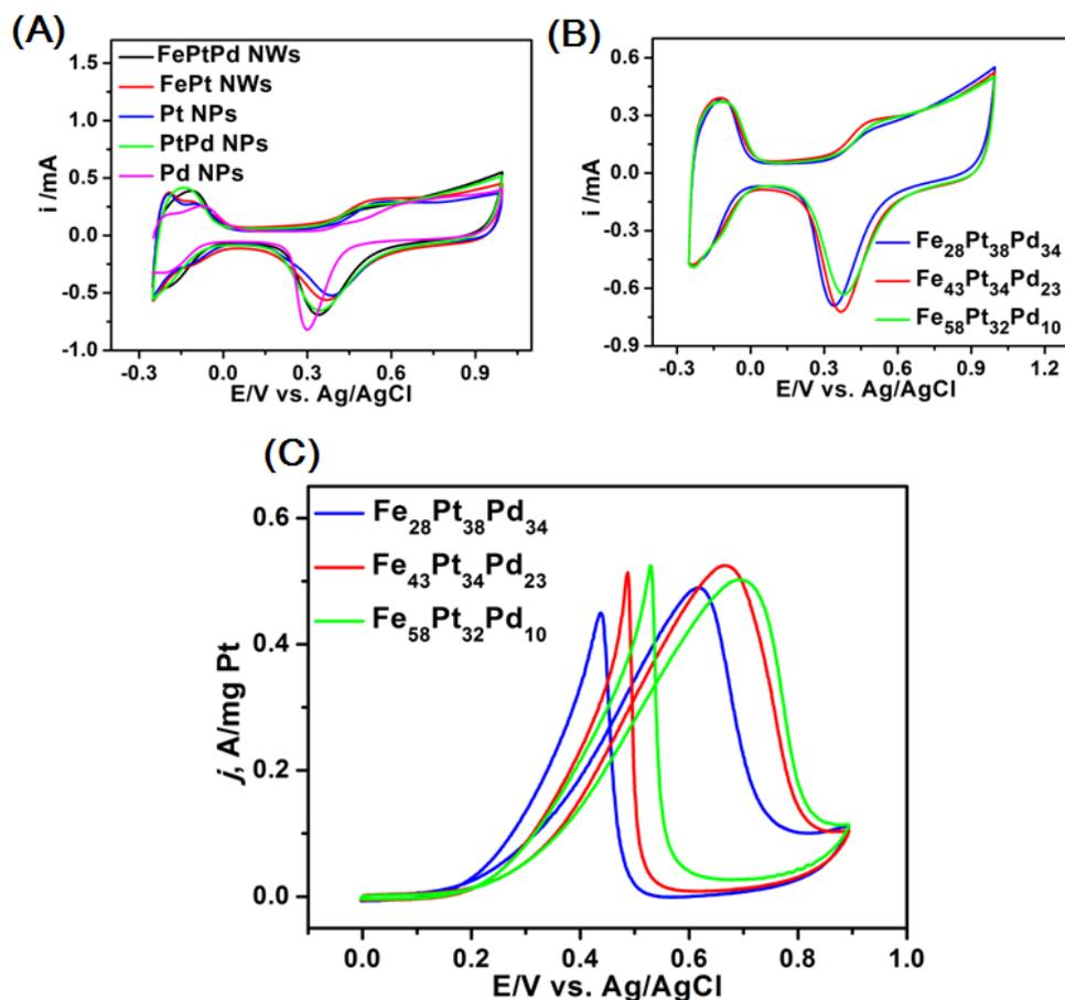
**Figure 8-5.** CVs of (A) Fe<sub>28</sub>Pt<sub>38</sub>Pd<sub>34</sub> NWs, FePt NWs, Pt NPs, Pd NPs and PtPd NPs and (B) FePtPd NWs with different compositions in N<sub>2</sub>-saturated 0.1 M HClO<sub>4</sub> solution at a scan rate of 50 mV/s. (C) CVs of MOR catalyzed by FePtPd NWs with different compositions in N<sub>2</sub>-saturated 0.1 M HClO<sub>4</sub> and 0.2 M methanol solution at a scan rate of 50 mV/s.
