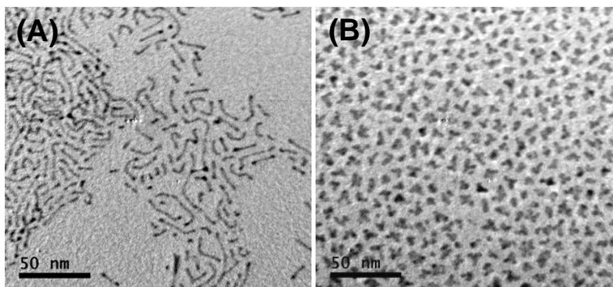
**Figure 8-3.** TEM images of (A) FePt NWs obtained at 160 °C and (B) the NPs obtained through adding  $\text{Fe}(\text{CO})_5$  into the mixture of  $\text{Pt}(\text{acac})_2$  and  $\text{Pd}(\text{acac})_2$ .
