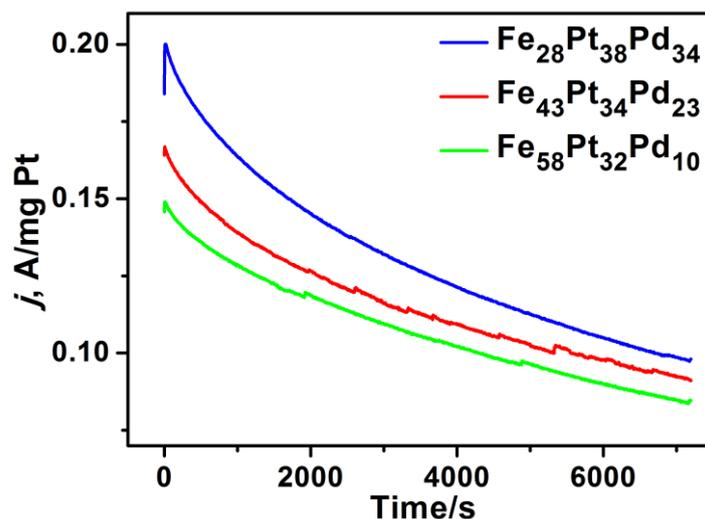
**Figure 8-8.** Current density-time curves of methanol oxidation reaction catalyzed by FePtPd NWs with different compositions in  $\text{N}_2$ -saturated 0.1 M  $\text{HClO}_4$  and 0.2 M methanol solution. The curves were collected at a constant potential of 0.4 V.
