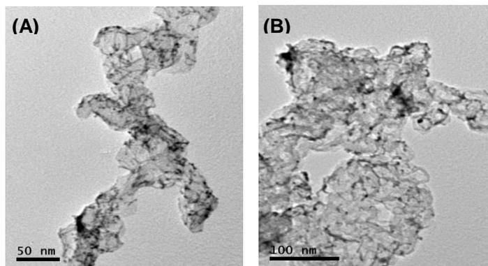
**Figure 8-9.** TEM images of the FePt NWs before (A) and after (B) 2 h i-t test.
