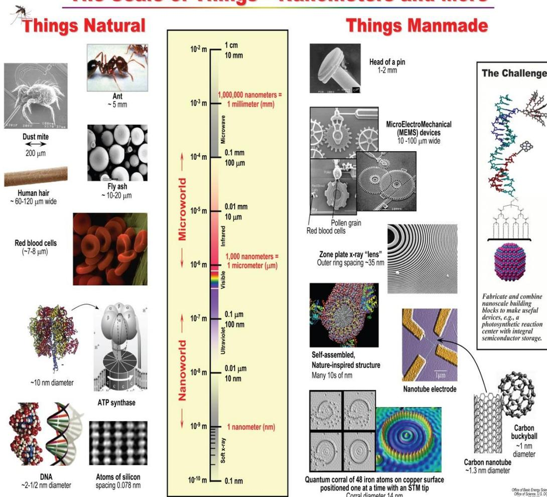
**Figure 1-1.** The scale of things to explain the regime of nanomaterials and the typical natural and artificial examples of nanomaterials. (Courtesy of the Office of Basic Energy Sciences, Office of Science, U.S. Department of Energy, [http://www.sc.doe.gov/bes/scale\\_of\\_things.html](http://www.sc.doe.gov/bes/scale_of_things.html))
