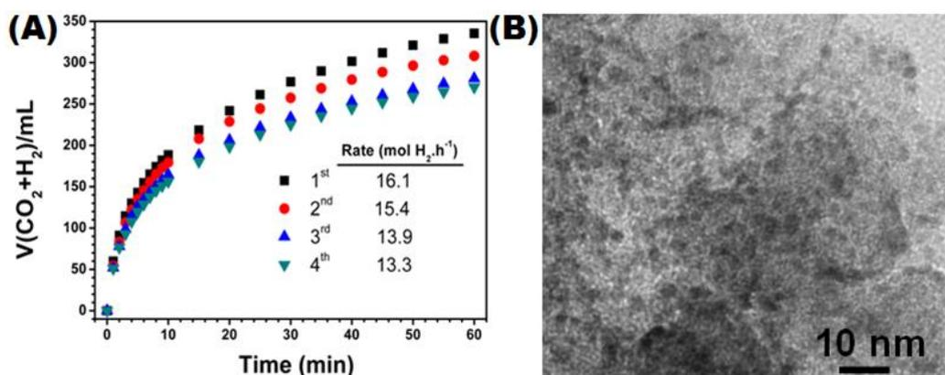
**Figure 9-12.** (A) The gas (CO<sub>2</sub>+H<sub>2</sub>) - reaction time plot obtained from four reaction cycles of the C-Ag<sub>42</sub>Pd<sub>58</sub> catalyst in the dehydrogenation of aqueous FA solution (10 mL, 1 M) at 50 °C. (B) A representative TEM image of the C-Ag<sub>42</sub>Pd<sub>58</sub> catalyst after the 4<sup>th</sup> catalytic run.
