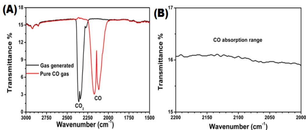
**Figure 9-8.** FTIR spectra of pure CO gas and gas generated during the C-Ag<sub>42</sub>Pd<sub>58</sub> catalyzed FA dehydrogenation in water at 50 °C for 1 h (**A**) and the zoom-in of the CO stretching absorption range (**B**).
