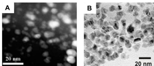
**Figure 9-2.** TEM images of AuPd NPs immobilized on metal organic framework and Ag/Pd core/shell NPs (Adopted from reference 5b and 8).
