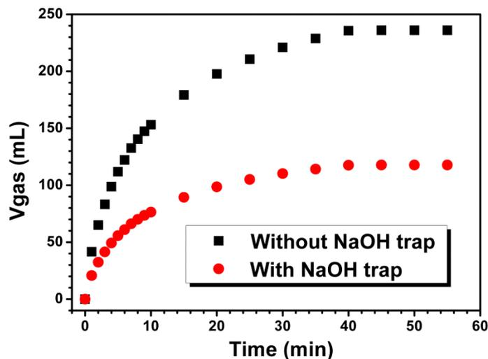
**Figure 9-9.** The comparison of the volume of gas generated during the C-Ag<sub>42</sub>Pd<sub>58</sub> catalyzed dehydrogenation of aqueous FA solution (10 mL, 0.5 M) with and without NaOH trap.
