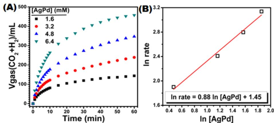
**Figure 9-10.** (A) Gas (CO<sub>2</sub>+H<sub>2</sub>) generated vs. time during the dehydrogenation of aqueous FA solution (10 mL, 1 M, 50 °C) in the presence of different catalyst concentrations, and (B) plot of hydrogen generation rate vs. AgPd concentration.
