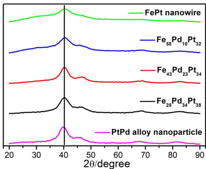
**Figure 8-2.** XRD patterns of PtPd NPs, FePt NWs and FePtPd NWs with different compositions.
