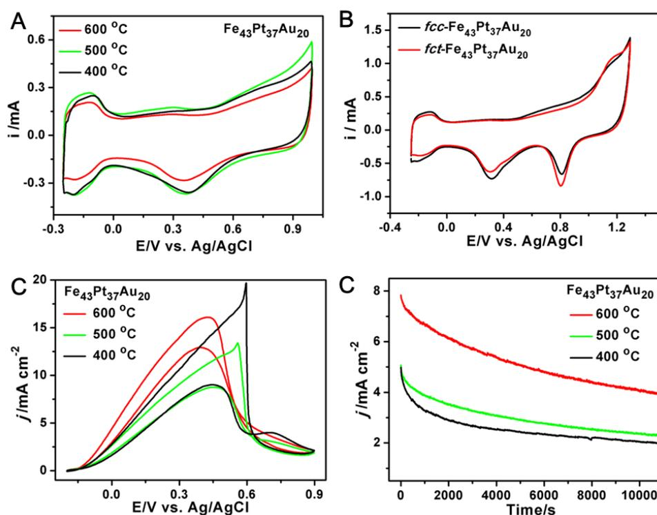
**Figure 7-7.** (A, B) CVs of the Fe<sub>43</sub>Pt<sub>37</sub>Au<sub>20</sub> NPs annealed at different temperatures with the
