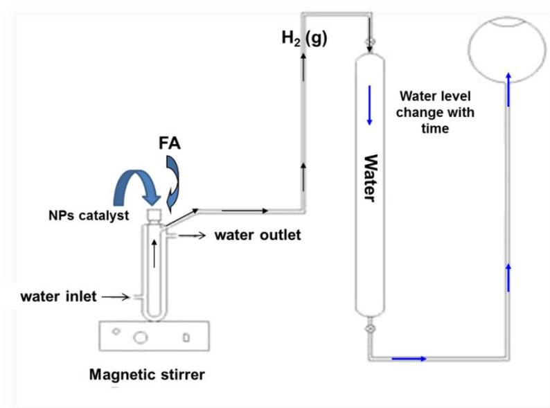
**Figure 1-7.** The illustration of the self-designed setup for FAD catalysis investigation.
