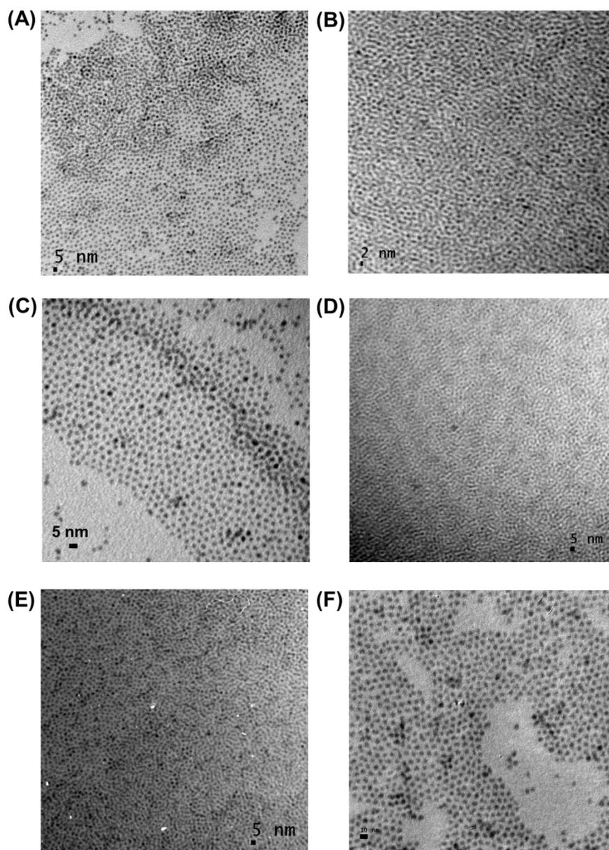
**Figure 9-4.** TEM images of (A) Ag<sub>25</sub>Pd<sub>75</sub>, (B) Ag<sub>52</sub>Pd<sub>48</sub>, (C) Ag<sub>60</sub>Pd<sub>40</sub>, (D) Ag<sub>80</sub>Pd<sub>20</sub>, (E) Ag NPs and (F) Pd NPs.
