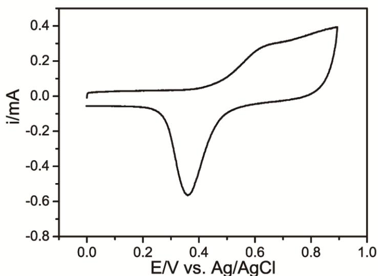
**Figure 8-6.** CV of methanol oxidation on a Pd/C-modified GC electrode in  $\text{N}_2$ -saturated 0.1 M  $\text{HClO}_4$  + 0.2 M methanol solution at the scan rate of 50 mV/s.
