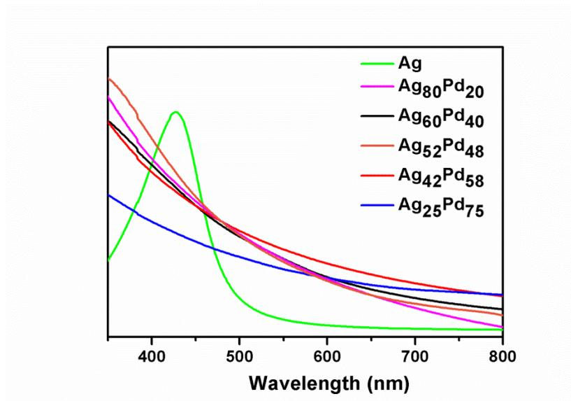
**Figure 9-6.** UV-vis spectra of the 2.2 nm Ag, Ag<sub>80</sub>Pd<sub>20</sub>, Ag<sub>60</sub>Pd<sub>40</sub>, Ag<sub>52</sub>Pd<sub>48</sub>, Ag<sub>42</sub>Pd<sub>58</sub> and Ag<sub>25</sub>Pd<sub>75</sub> NPs.
