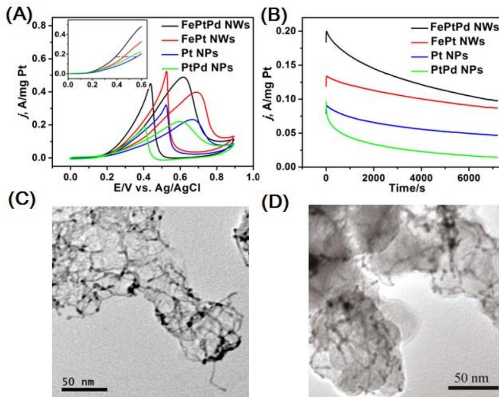
**Figure 8-7.** CVs (A), linear sweep voltammetry (inset) and i-t curves (B) of MOR catalyzed by  $\text{Fe}_{28}\text{Pt}_{38}\text{Pd}_{34}$  NWs, FePt NWs, Pt NPs and PtPd NPs in 0.1 M  $\text{HClO}_4$  + 0.2 M methanol solution. The CVs were obtained at a scan rate of 50 mV/s and the i-t curves were collected at a constant potential of 0.4 V. TEM images of the  $\text{Fe}_{28}\text{Pt}_{38}\text{Pd}_{34}$  NWs/C before (C) and after (D) 2 h i-t test.
