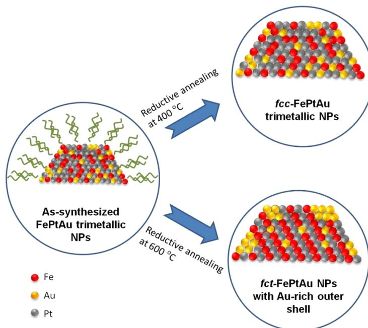
**Figure 7-5.** Schematic illustration of the structural change of the FePtAu NPs upon annealing. When annealed at 400 °C, the FePtAu NPs are *fcc* structured, but at 600 °C, the *fct*-FePtAu structure is formed with Au-segregating on the NP surface.
