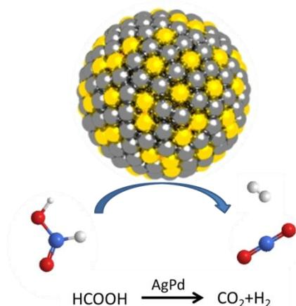
**Figure 9-1.** The schematic illustration of FA dehydrogenation catalyzed by NP heterogeneous catalyst.
