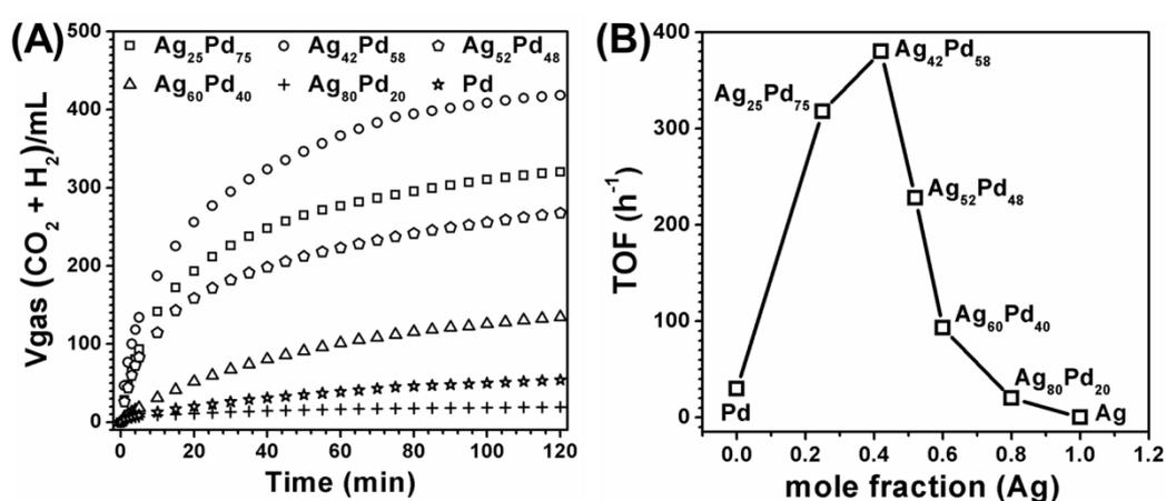
**Figure 9-7.** (A) The plots of gas (CO<sub>2</sub>+H<sub>2</sub>) generated vs. time during the dehydrogenation of aqueous FA solution (10 mL of 1 M, 50 °C) in the presence of C-AgPd and C-Pd catalysts and (B) TOF vs. mole fraction of Ag for the C-AgPd catalysts at different Ag, Pd compositions.
