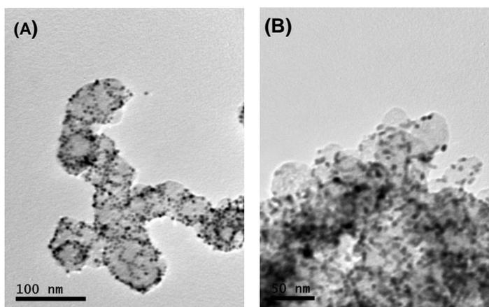
**Figure 8-10.** TEM images of the Pt NPs before (A) and after (B) 2 h i-t test.
