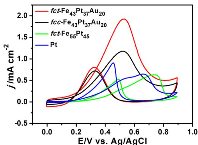
**Figure 7-10.** CVs of the *fct*-Fe<sub>43</sub>Pt<sub>37</sub>Au<sub>20</sub>, *fcc*-Fe<sub>43</sub>Pt<sub>37</sub>Au<sub>20</sub>, *fct*-Fe<sub>55</sub>Pt<sub>45</sub> and commercial Pt NPs in the N<sub>2</sub>-saturated 0.5 M H<sub>2</sub>SO<sub>4</sub> and 0.5 M methanol solution.
