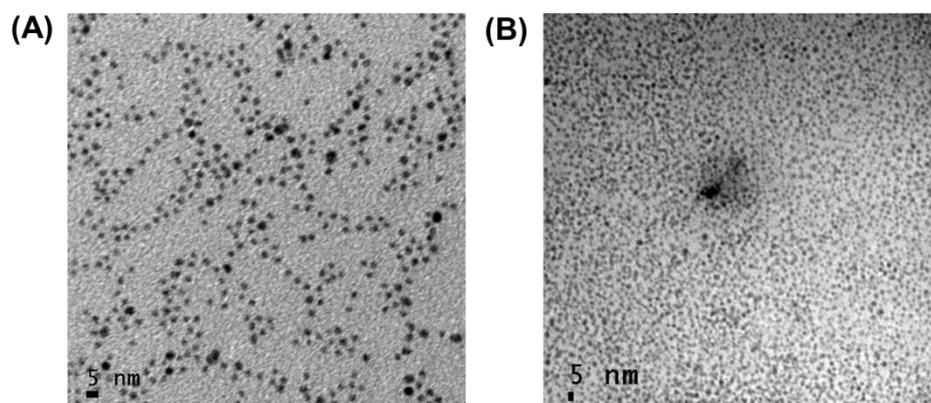
**Figure 9-5.** TEM images of the AgPd NPs synthesized by using (A) 0.5 ml of OA and (B) without OA.
