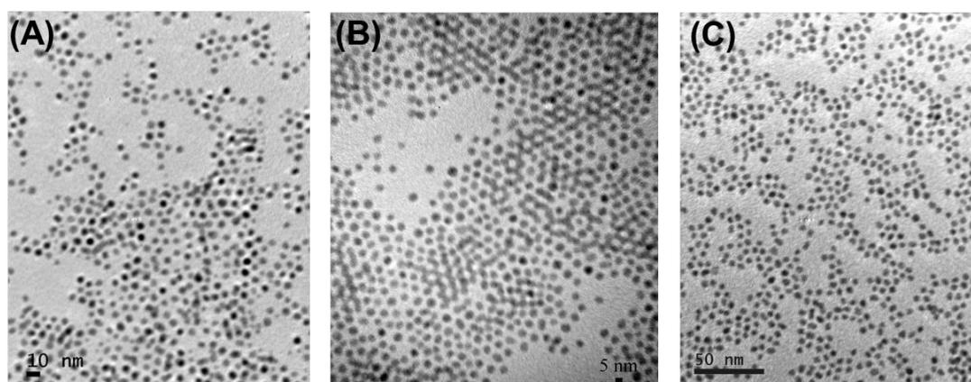
**Figure 8-4.** TEM images of (A) 3 nm Pt NPs, (B) 5 nm Pd NPs and (C) 4 nm PdPt NPs.
