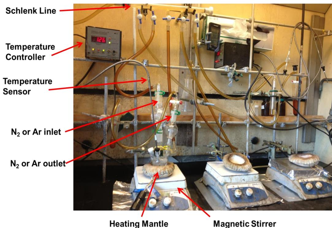
**Figure 2-2.** General set-up used to synthesize NPs in Sun group. Picture was taken in Geochem 309 with permission from Sun group.
