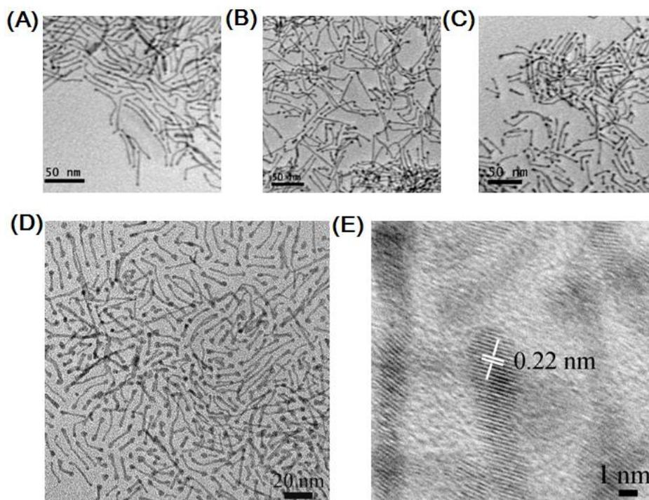
**Figure 8-1.** TEM (A-D) and HRTEM (E) images of  $\text{Fe}_{68}\text{Pt}_{32}$  (A),  $\text{Fe}_{58}\text{Pt}_{32}\text{Pd}_{10}$  (B),  $\text{Fe}_{43}\text{Pt}_{34}\text{Pd}_{23}$  (C) and  $\text{Fe}_{28}\text{Pt}_{38}\text{Pd}_{34}$  NWs (D, E).
