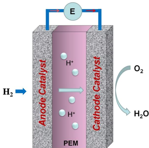
**Figure 1-3.** Schematic illustration of a typical PEMFC with  $H_2$  as fuel.
