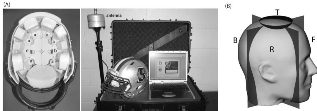
Figure B.1: Football players wore helmets instrumented with the HIT system that was specifically designed to record head accelerations as a result of an impact to the helmet without interfering with play. The HIT System (A) is comprised of an in-helmet unit containing six accelerometers (a), battery (b), transmitting and logging electronics (e), a sideline receiver, and a laptop computer. An illustration of the regions that defined the front (F), right side (R), back (B) and top (T) helmet impact locations (B) .
