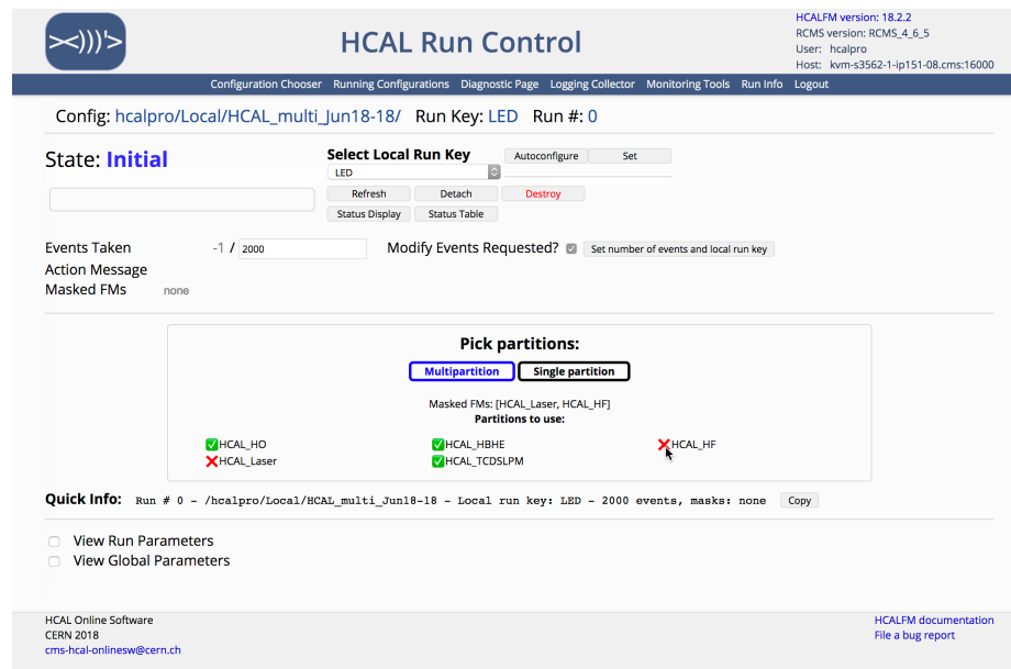
Figure A.5: A screen capture of the HCALFM graphical user interface showing the multipartition masking panel.
