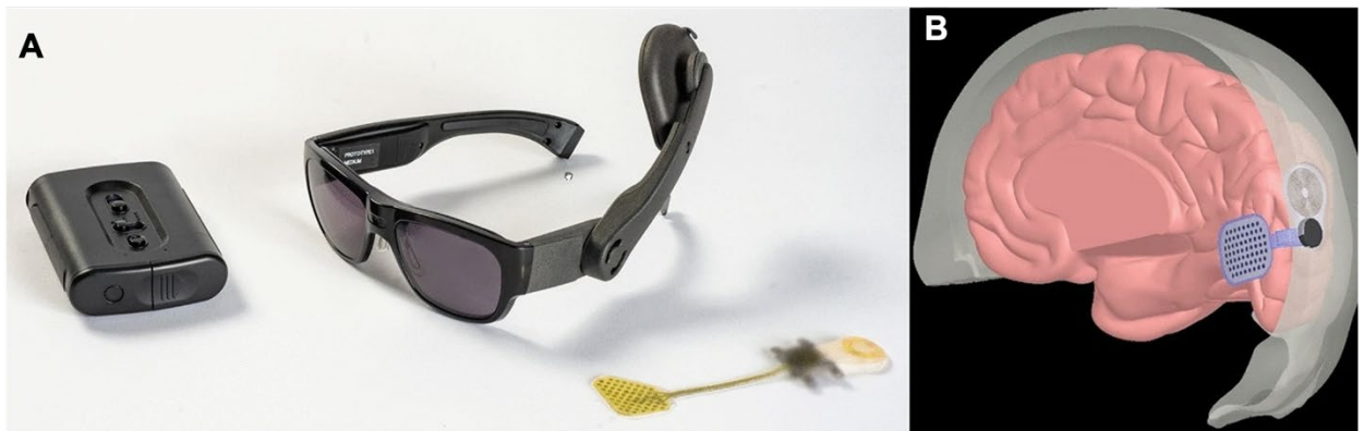
Figure 4 (A) Image of the external portion of the ORION cortical implant shown alongside the cortical implant in the right corner of the image, (B) location of the ORION implant in the visual cortex. Adapted from Ramirez et al., 2023 [20] .
