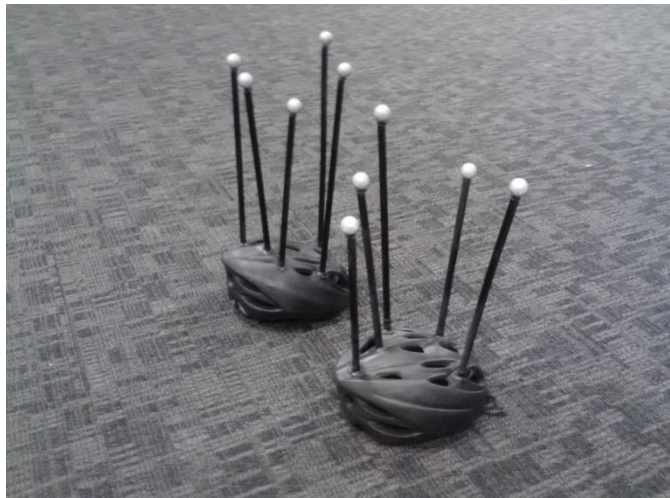
Figure 7-1: Two helmets worn by participants in Experiment 4. Each helmet was outfitted with five reflective markers on protruding stalks to create a unique 'constellation' that could be detected and tracked.
