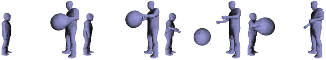
Figure 4.1: Mesh based representation by Arcila et al. [8]. Here mesh connectivity is unable to deal with changing scene topology
