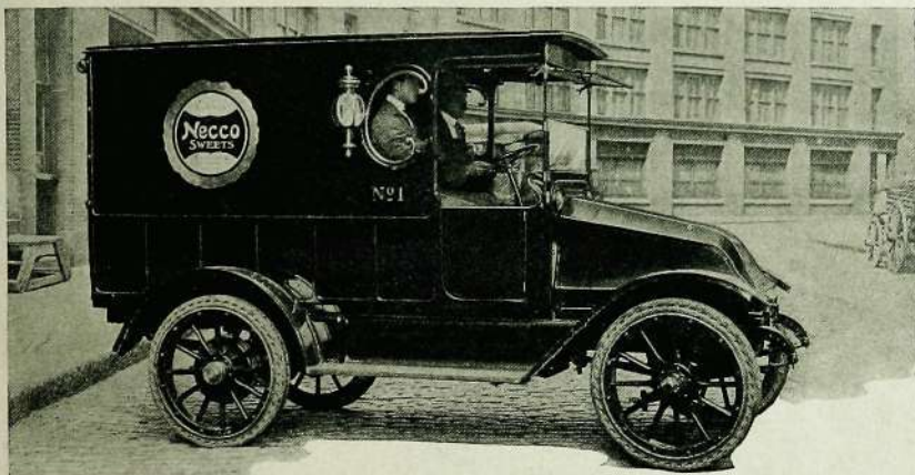
(One of the 4,000 G. V. Electrics out on the firing-line. A 1,000-lb. wagon, worm-drive type. Speed 12 to 15 miles per hour; 45 to 65 miles per battery charge.)
