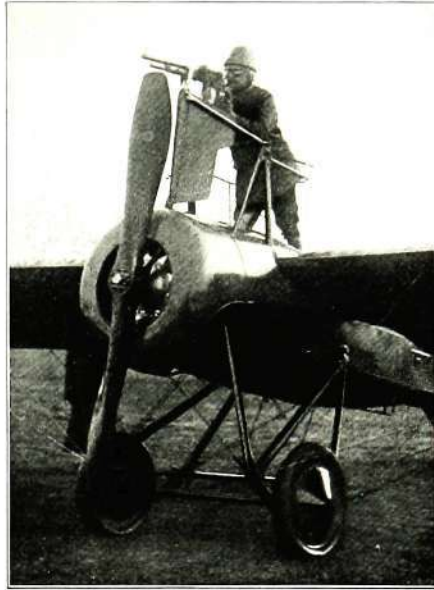
French armored monoplane with a Hotchkiss rapid-fire gun.
