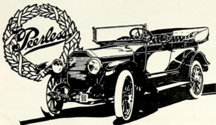
Peerless "All-Purpose" Six. Wheel-base 121 inches. Weight 3000 pounds.
