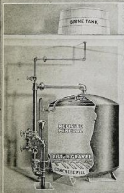
Sectional View of Refinite Water Softener
