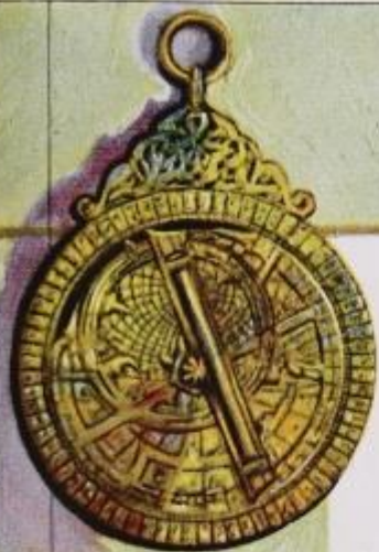
An astrolabe of the XIII th. Century. This instrument was introduced into Europe by the Arabs about 700 A.D. Aptly termed "the mathematical jewel", it was used in making astronomical cal- culations; also in determining time.
