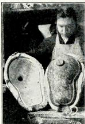
Left.—Pouring the glue (or gelatine) into the shell and around the head which is inside. Centre.—The shell open, showing the gelatine, which has set. The original model has been removed and the space it occupied filled with plaster of paris and water. Right.—The plaster has set, and the gelatine mould is being pulled off. Notice its flexibility. Several plaster copies can be made from this mould.
