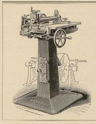
LINING-BEVELERS are intended to do that perfect work on a Photo-engraved plate that the brain can conceive, but the hand can not execute. They will carry out the idea of the artist in framing or making a finished border that completes the lines of the picture.
