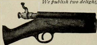
Showing Position of Ejector in Ejecting Shell.
