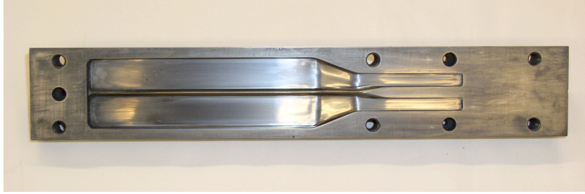
Figure 3.2. Mold for growing bicrystals. Note the two compartments for housing single crystal seeds.
