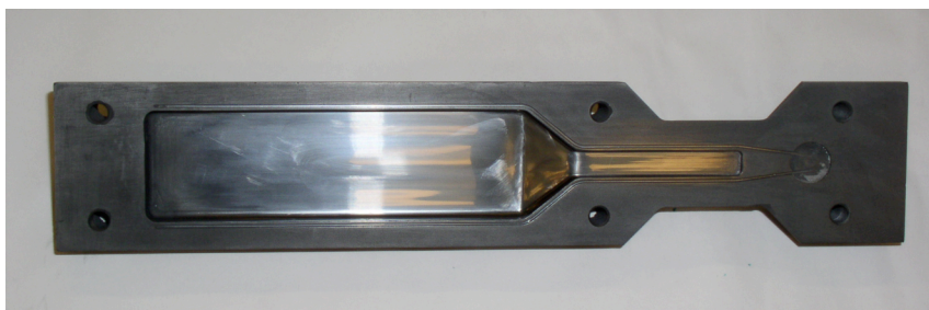
Figure 3.1. Split graphite mold for single crystal growth using the vertical Bridgman method.
