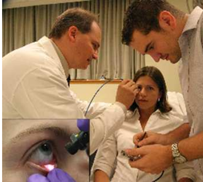
Figure 4.22: Photograph of data collection using fiber optic probe and collinear collection/irradiation fibers.
