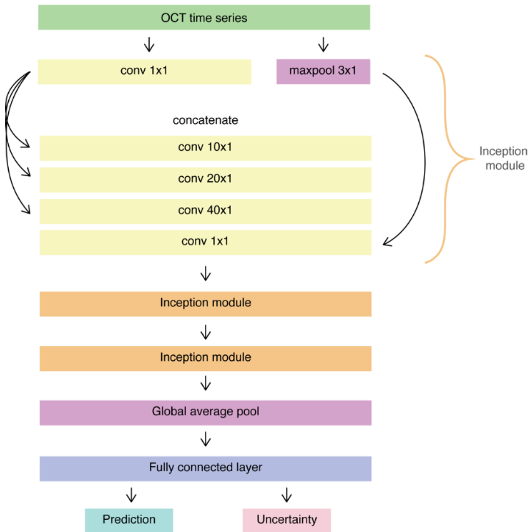
Supplementary Figure 5.6. InceptionTime 1D CNN architecture for the prediction of RBC flux from OCT time series data.
