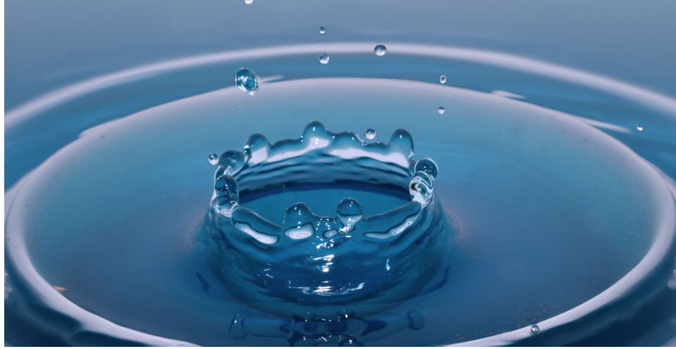
Figure B.1: Worthington-Edgerton crown created by a droplet impacting the free surface of a stagnant liquid.
