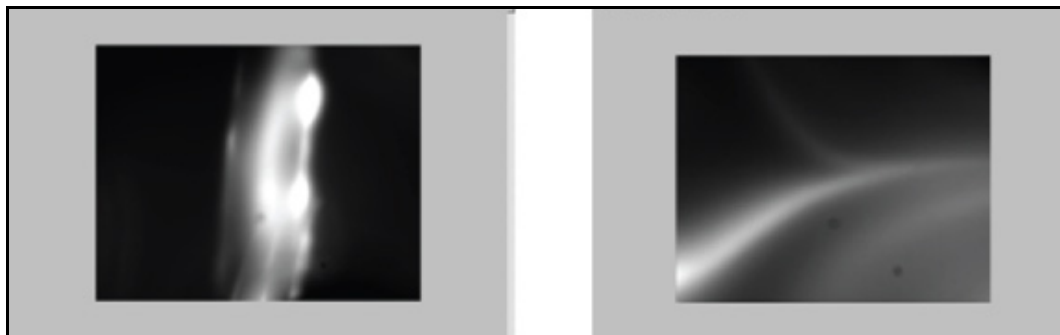
Figure 26: Fluorescent microscope images of DNA in the “starting line” chip. Left: DNA concentrated on the positively-biased platinum wire. Right: DNA being released or “launched” when a negative potential is applied to the platinum wire.
