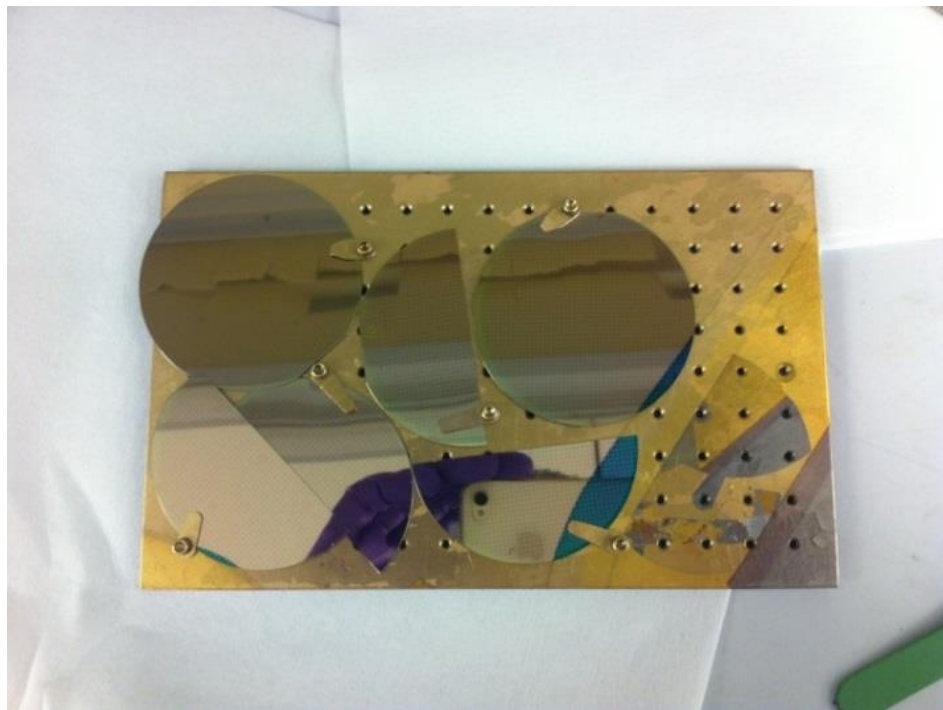
Fig. 2.8: Example of wafer arrangement for E-beam evaporation deposition
