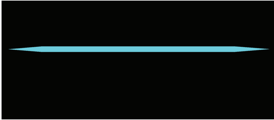
Figure A.2: Bitmap image of the pre-crack template. The RGB values at every pixel prescribe the dwell time (0..255) for the ion mill; black areas correspond to no milling involved.
