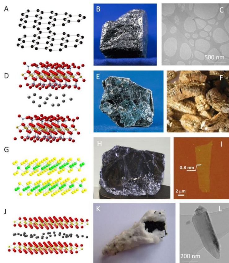
Figure 1-7 Ball-and-stick model of crystal structures, naturally occurring forms, and exfoliated nanosheets for four example layered materials (A-C: graphite/graphene; D-F: layered silicate hydrate; G-I Molybdenite/Molybdenum disulfide; J-L: Birnessite/Manganese dioxide) Image reproduced from [98].
